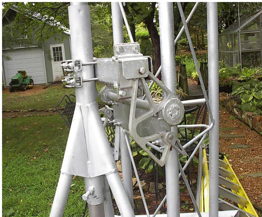
The photo below shows the rotor mounted in place ready for an antenna mast. The last photo below shows and antenna in place on the hazer shelf ready to be hoisted in the air!
